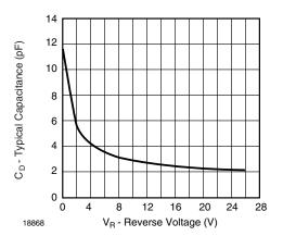
Figure 2. Typical Capacitance vs. Reverse Applied Voltage
